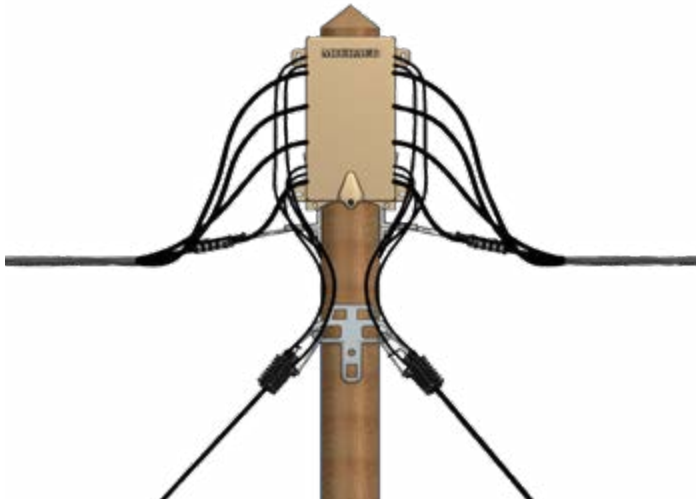
Network junction + service connections
